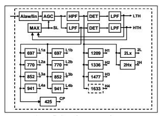
Figure 5: Complete DTMF detector
