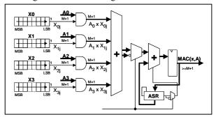
Figure 6: Serial MAC (picture based on [5])
