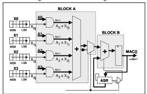
Figure 7: Serial MAC using ALTERA (based on [5])
