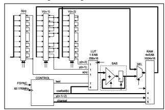
**Figure 8**:. Goertzel Coprocessor for DTMF detection These building blocks operate as follows:
