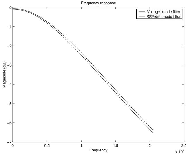
Figure 11: HSPICE simulations of the adjoint lowpass filters with a cut-off frequency of 1MHz.
