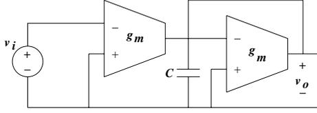
Figure 2: *OTA-C* filter working in voltage mode.
