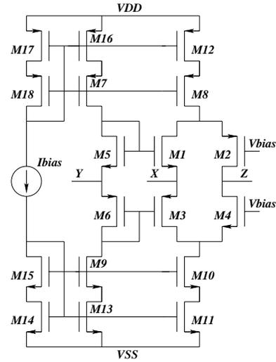
Figure 6: CCII- designed with CMOS technology
