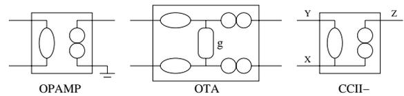
Figure 1: Basic nullor-based analog building blocks.
