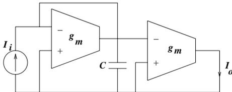
Figure 4: *OTA - C* filter working in current mode.
