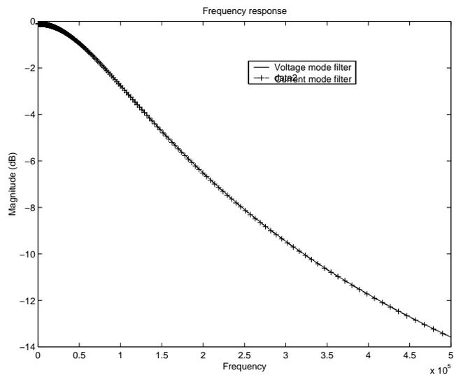
Figure 10: HSPICE simulations of the adjoint lowpass filters with a cut-off frequency of  $100\text{kHz}$ .
