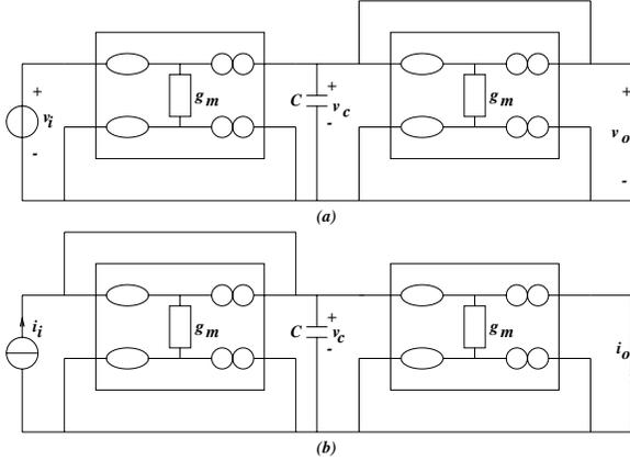
Figure 3: Nullor-based *OTA-C* filter working in (a) voltage and (b) current mode.
