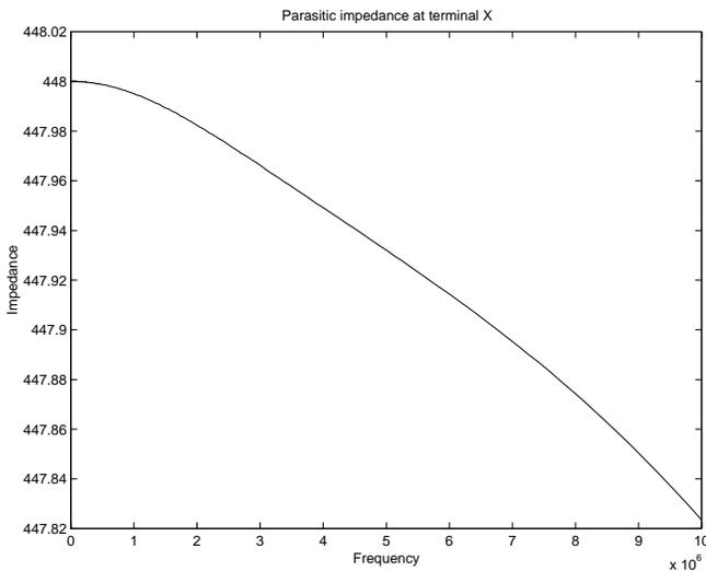
Figure 8: Parasitic impedance of the CCII- at node X.
