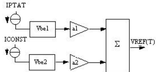
Fig.1 Block diagram of the curvature-corrected bandgap type circuit
