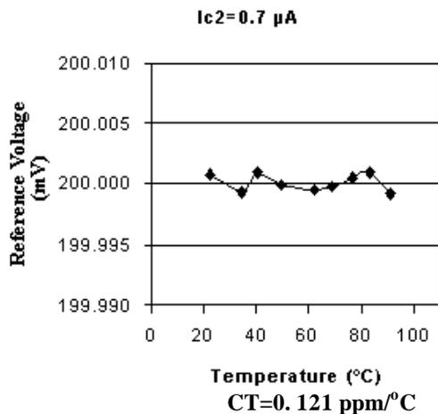
Fig. 4 Variation of  $V_{REF}(T)$  with temperature for device MAT01 #1
