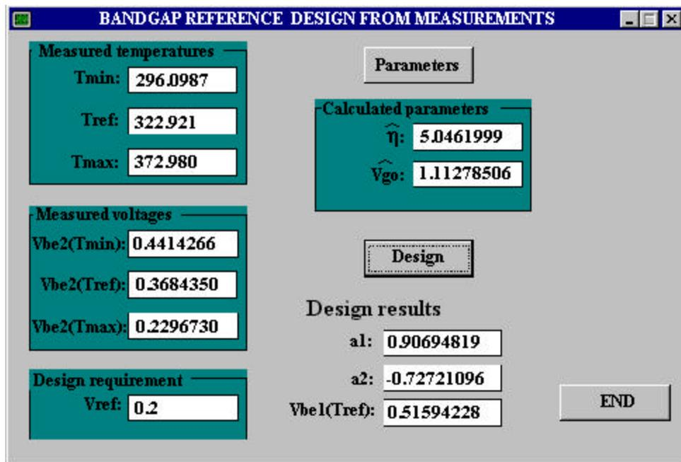
Fig.3 Program screen with design results for MAT01#1.
