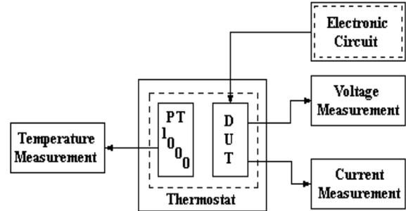
Fig.2 Block diagram of the measurement setup
