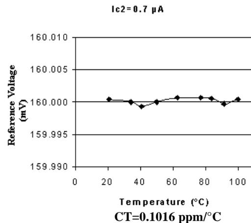
Fig.5 Variation of  $V_{REF}(T)$  with temperature for CMOS substrate PNP # N1202
